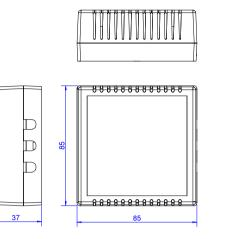
The instrument is based on fully calibrated, linearised and temperature compensated semiconducting metal-oxide gas sensor with high repeatability, stability and long lifetime. The sensor exhibits high selectivity to common volatile solvents, as ethanol, toluene, xylene etc.
