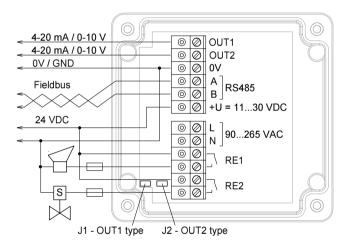
To use analog outputs, connect the terminals **OUT1** and/or **OUT2** and **0V** to the input of the secondary instrument (indicator or controller). NB! The outputs are not galvanically isolated from 24 V power supply and share common 0V. Allowed load resistance limits are stated in Specifications table.
